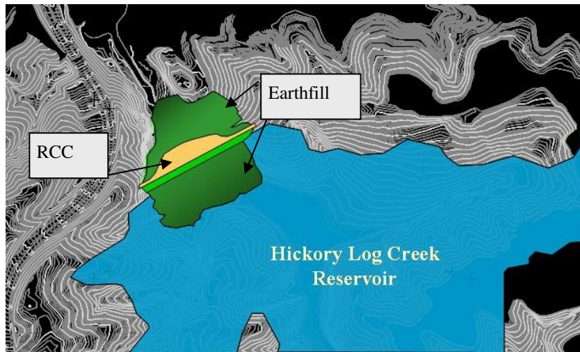
Figure 2. Earthfill versus RCC Dam Footprints
